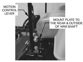
FIGURE 5 CONTROL ARM SHAFT
